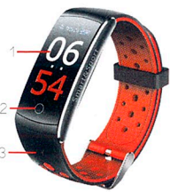
1. TFT Display 2. Touch area 3. Watch strap
